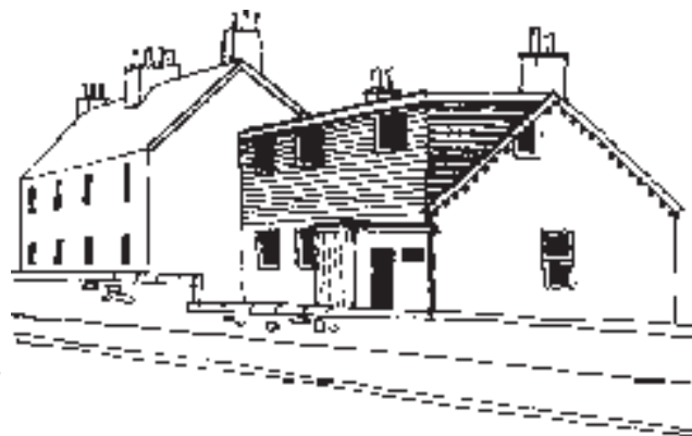
Overlarge and dominating dormer built off wall head.
